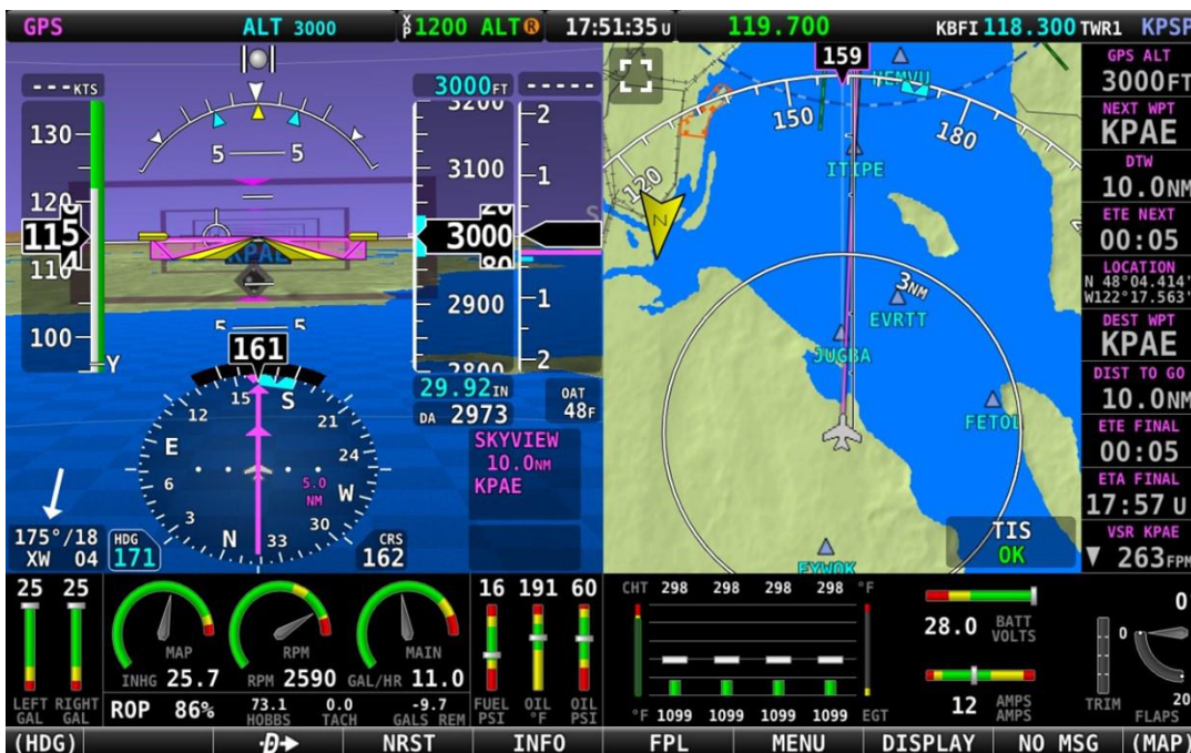
Figure 145: MAP/HSI with Navigation active
