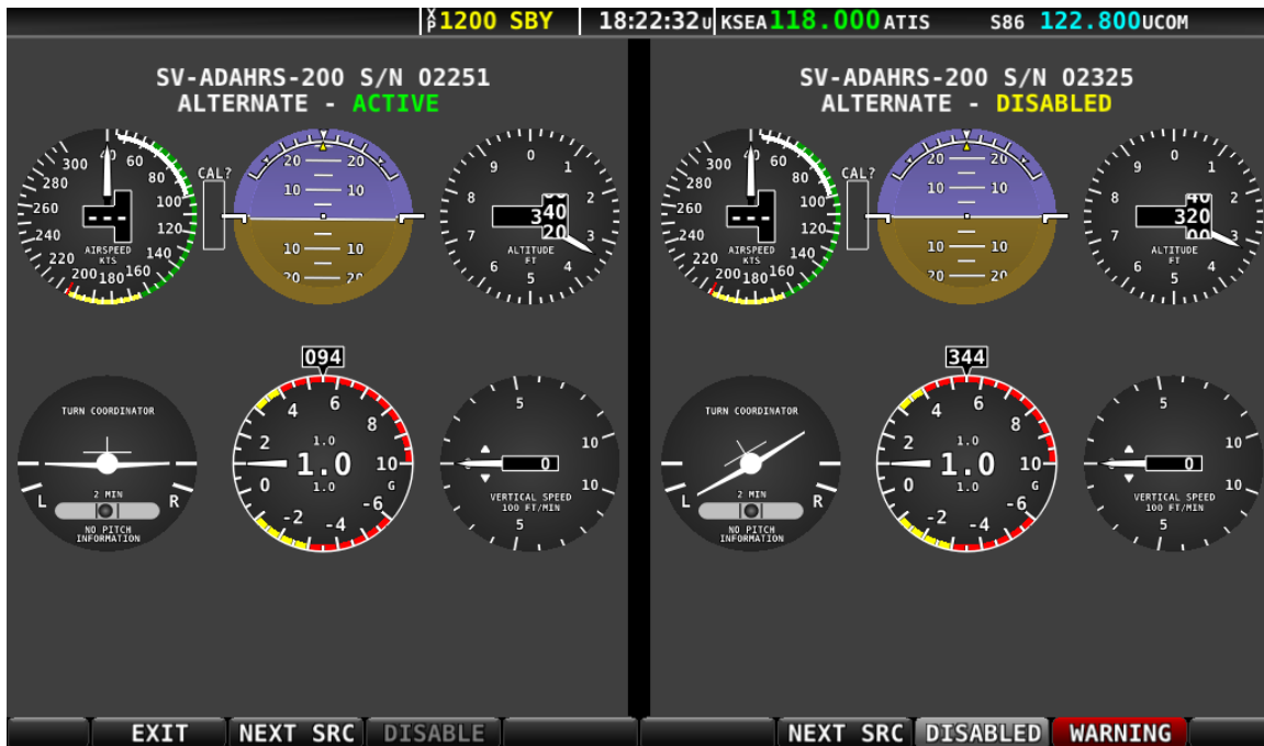
Figure 90: ADAHRS cross-check comparison (Six Pack presentation).
