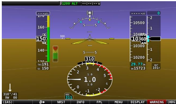
Figure 80: G Meter in EFIS Presentation PFD
