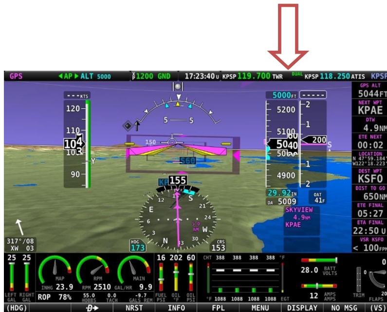
Figure 241: SkyView Top Bar Com Radio status overview
