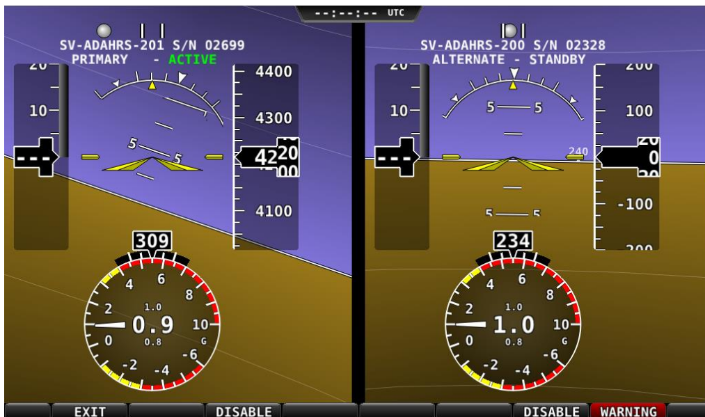
Figure 88 – ADAHRS Cross-Check Comparison (EFIS Presentation)
