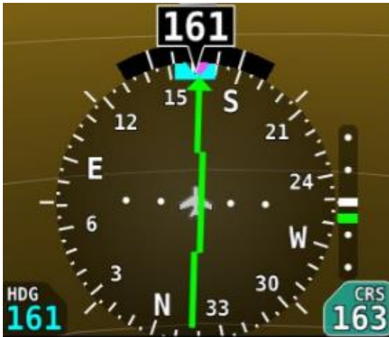
Figure 42: HSI example: Localizer
