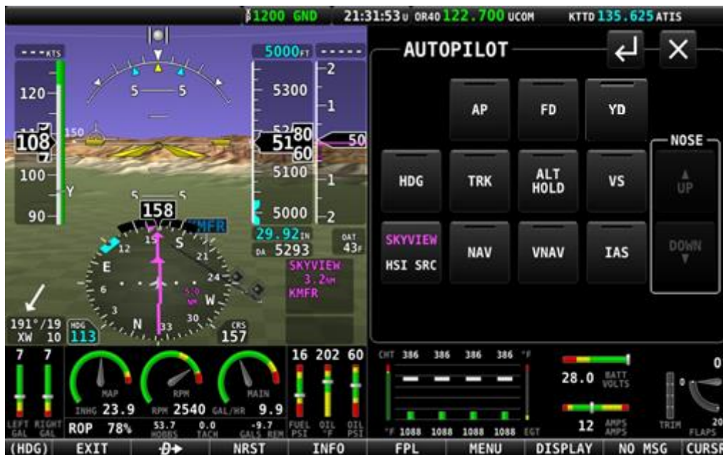
Figure 229: AUTOPILOT Page – Expert Control Scheme
