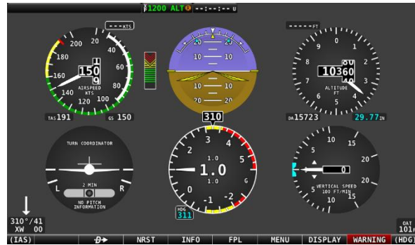
Figure 79: G Meter in Six-Pack Presentation PFD
