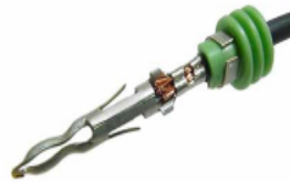
Figure 76 – Detail view of properly crimped pin.
