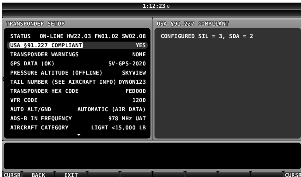
Figure 171 - 14 CFR § 91.227 Compliance Status – Compliant
