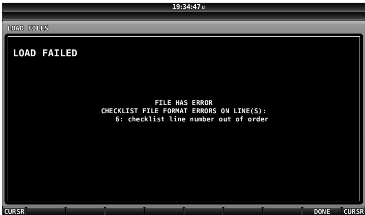
Figure 267 – Checklist File Has an Error, Line Number Displayed, Could Not Be Loaded
