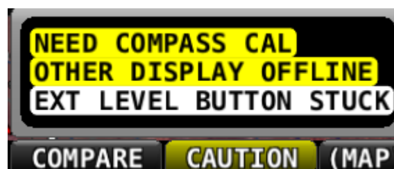
Figure 148 – EXT LEVEL BUTTON STUCK Message
