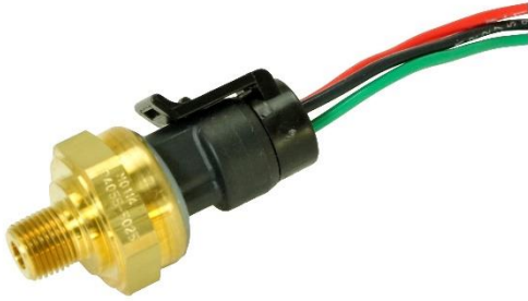
Figure 93 – Original 1/8-27 NPT 0-15 PSI Sensor (P/N 101690-000)
