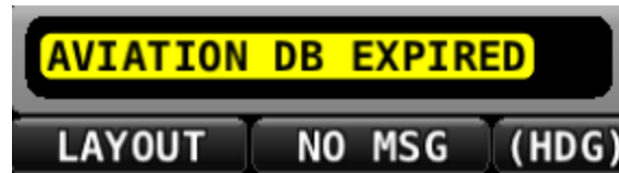
Figure 61 – SkyView SE Aviation Database Expired Caution Message (Lower Left Corner of Display)
