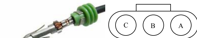
Figure 3: Pin insertion (rear) view of supplied connector.
